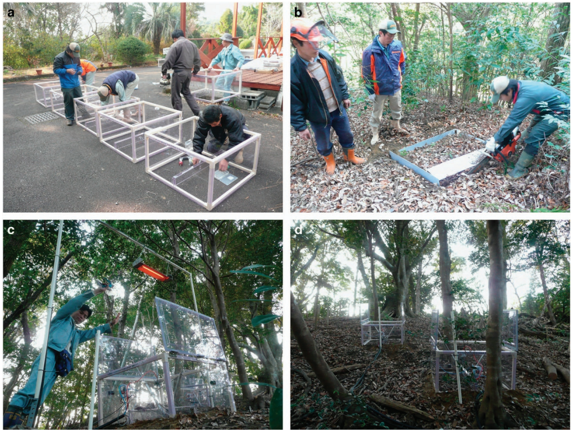
Figure 3. Chamber system installation at the Miyazaki Experimental Warming Site. (a) The chambers were assembled in the field. (b) Trenches were created using a chainsaw to sever roots. (c) The carbon-filament heat lamp was installed above the warming chamber. (d) Photograph of the study site with the chambers installed. The authors affirm that the individuals depicted herein provided informed consent for the use of their images.
