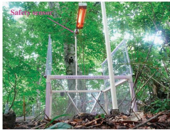
Figure 2. The infrared carbon-filament heat lamp was coupled with a safety sensor during the soil warming experiment in forest to reduce the risk of fire.
