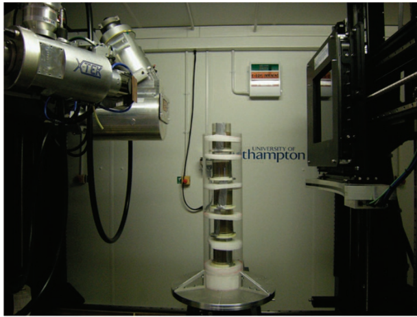
Figure 1. Five aquaria stacked in the holding brace in the micro-focus computed tomography scanner housed within the \mu -VIS X-ray Imaging Centre, University of Southampton.
