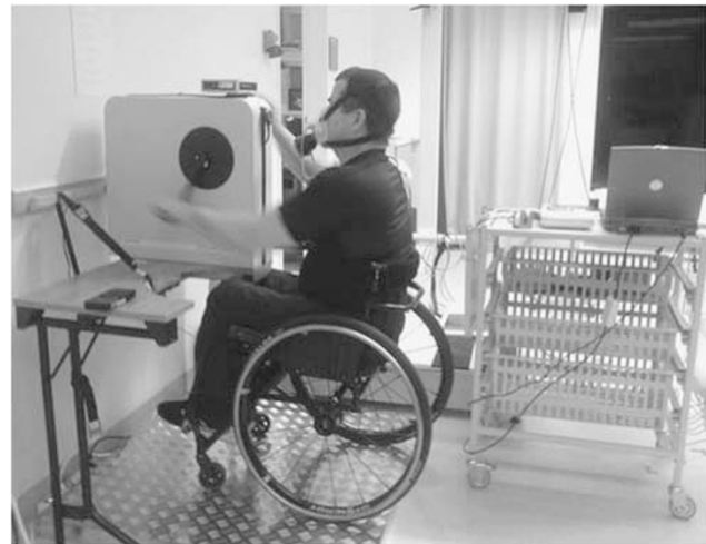
Figure 1 Setup for testing maximal oxygen uptake during ACE and ACE combined with LEVO.
