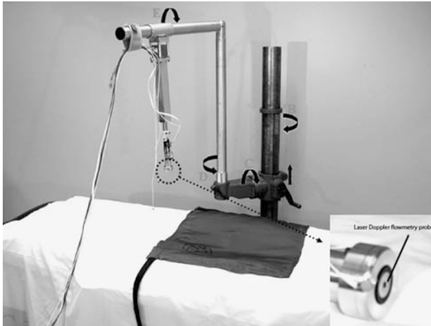
Figure 1 Photograph of the computer-controlled indenter system with a compound sensor head, positioning table and pressure mapping system A, B, C, D and E shown in the figure indicate the degrees of freedom for adjustment. The laser Doppler flowmetry probe is embedded in the central area of the indenter head.
