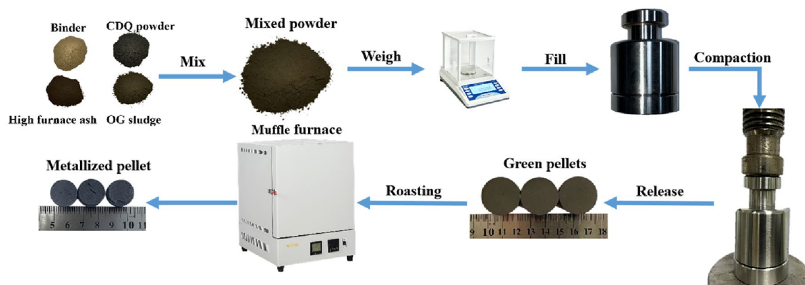
Figure 2. Preparation process of metallized pellets.
