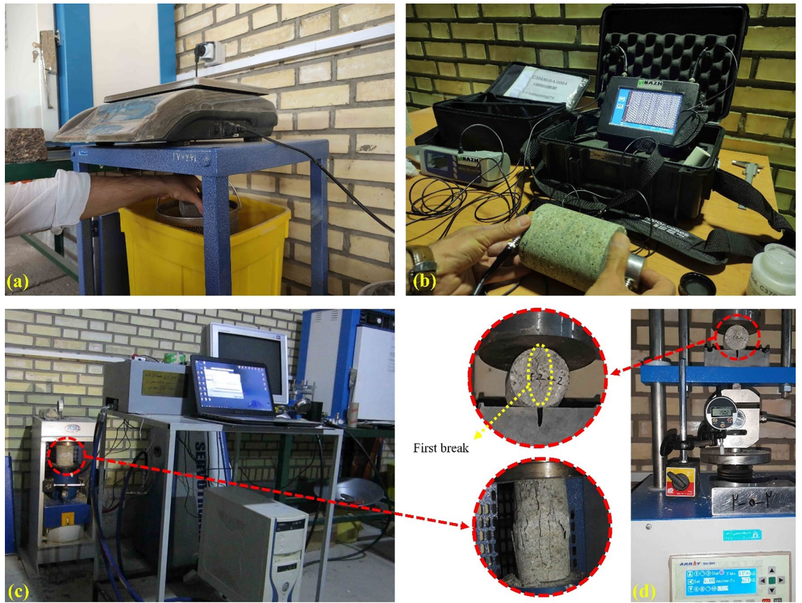
Figure 6. A view of the setup and testing methods, (a) physical property tests, (b) ultrasonic pulse velocity tests, (c) uniaxial compressive strength tests, (d) splitting tensile strength tests.
