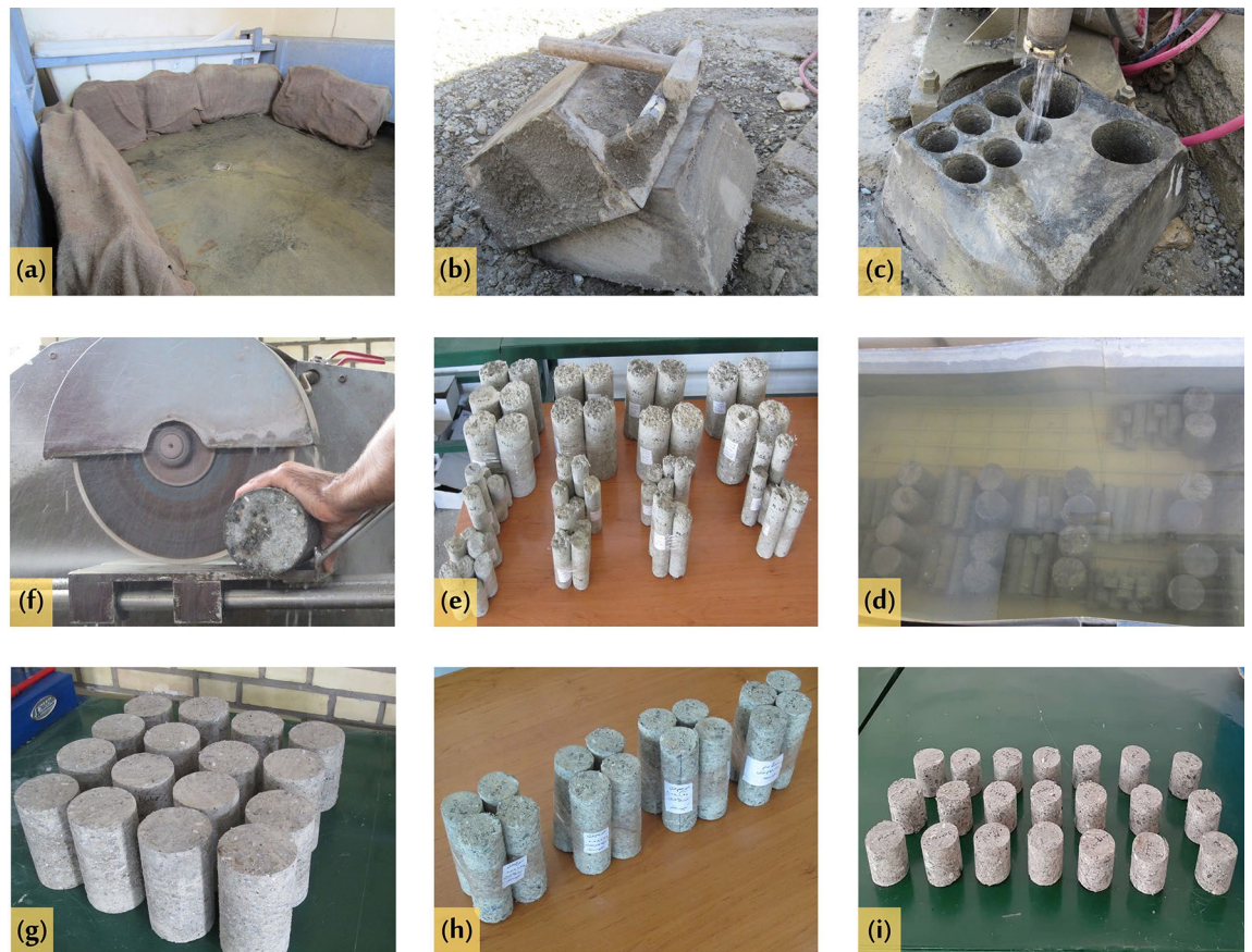
Figure 5. Sample preparation operations, (a) tissue-covered panels in curing room, (b) removing the panels from molds, (c) samples coring operation, (d) immersing the samples in water, (e) transferring the samples to the laboratory, (f) cutting the samples end, (g) prepared samples for uniaxial compressive strength and ultrasonic pulse velocity tests, (h) prepared samples for physical properties tests, (i) prepared samples for splitting tensile strength tests.
