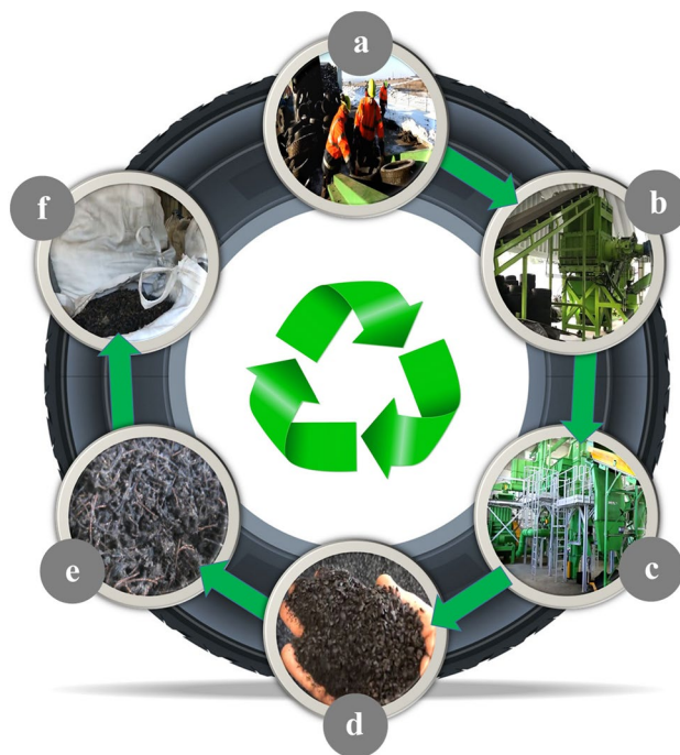
Figure 2. Treatment process of end-of-life-tires, (a) gathering the ELTs, (b) shredding operation, (c) separating the generated components by applying suction, (d) rubber powder, (e) waste tire textile fiber, (f) compacting and packing the WTTFs.
