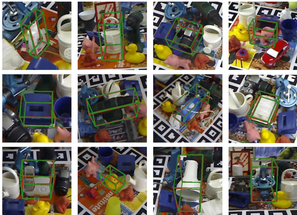
Figure 8. Results on the LINEMOD dataset. The green 3D bounding boxes denote the results of the proposed method; the red 3D bounding boxes represent the ground truth.
