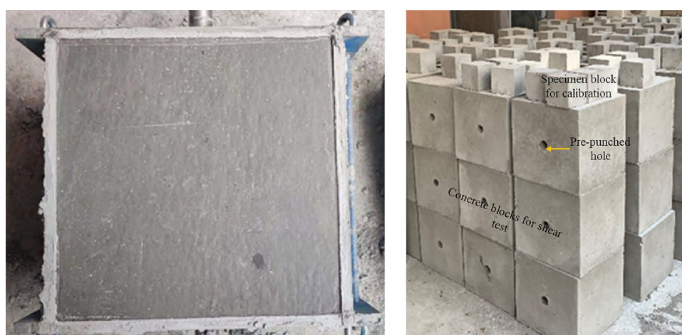
Figure 2. Fabrication of concrete blocks.
