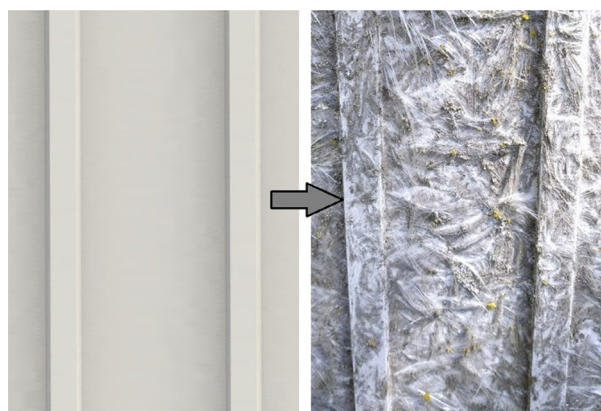
Figure 1. Degradation of the fiber-reinforced polymer composite after ten years of environmental exposure (electrical device housing).
