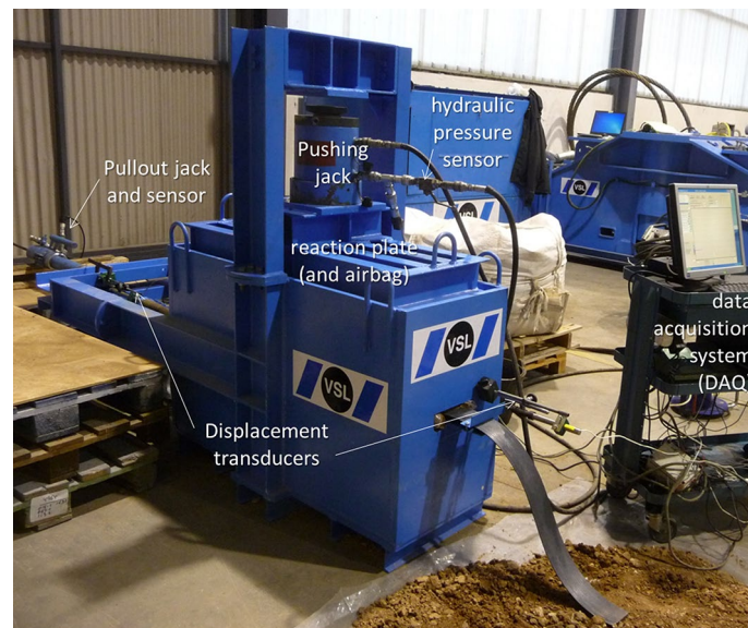
Figure 2. Pullout test box setup and main components.
