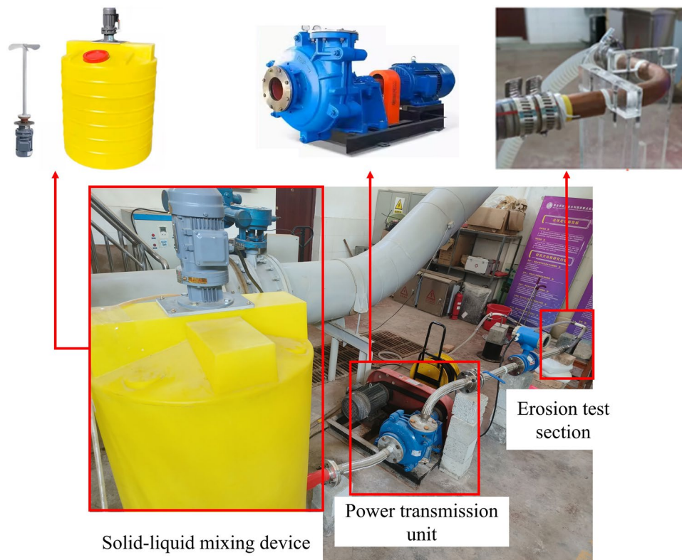
Figure 3. Water-cooled radiator pipe erosion and wear test bench.
