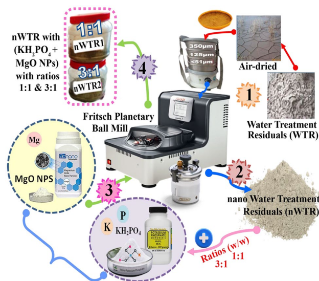
Figure 1. Schematic diagram of synthesis steps of nano-enabled fertilizers (NEF) based water treatment residuals nanoparticles (nWTR).
