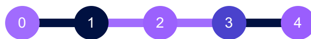
Figure 5. Qubit topology of 5-qubit ibmq_santiago v1.3.40 and ibmq_manila v1.0.19 devices. The colours of the qubits represent the frequency, with darker meaning a lower frequency and lighter meaning a higher value.
