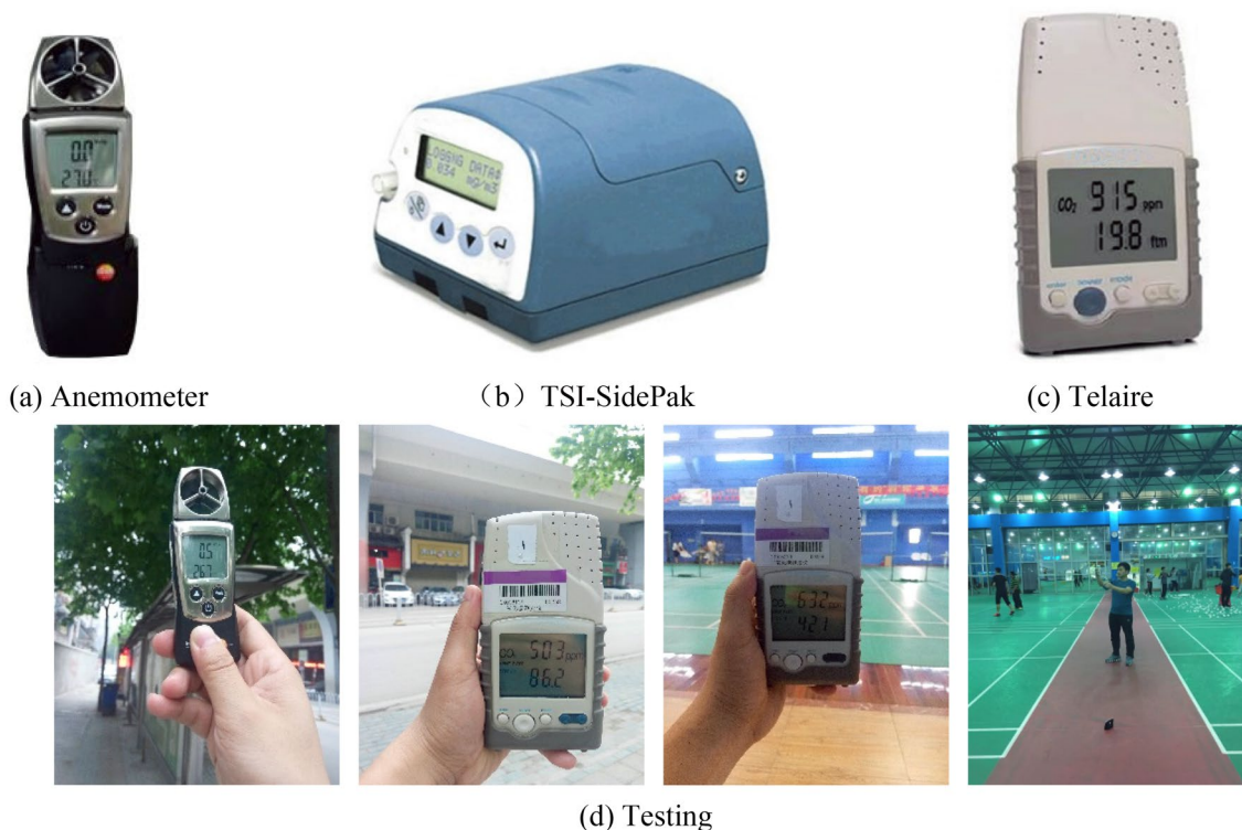
Figure 3. Testing instruments (a, b, c); Testing (d).
