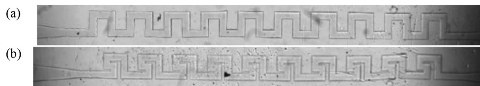
Figure 3. Images of the (a) square wave microchannel and (b) modified square wave microchannel.
