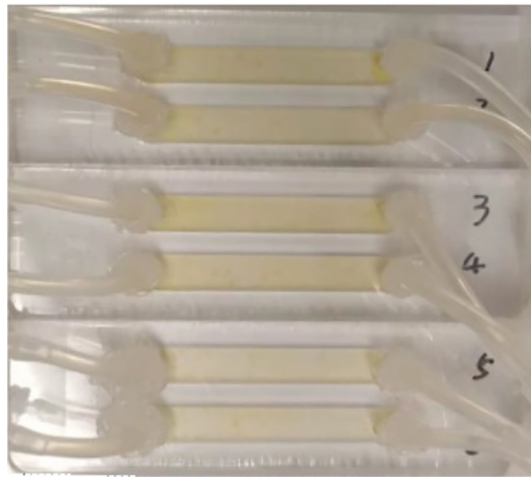
Figure 7. Custom-made flow-cell with C. vulgaris biofilms growing inside. Each one has two separated channels.
