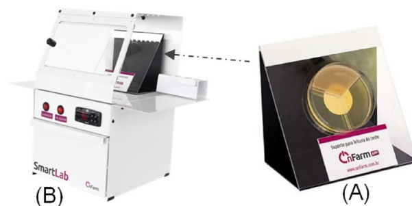
Figure 1. Reader Support (A) located at the SmartLab Incubator (B; OnFarm, Piracicaba, São Paulo, Brazil) used to take pictures for model training and performance evaluation. Source: OnFarm (Piracicaba, São Paulo, Brazil).
