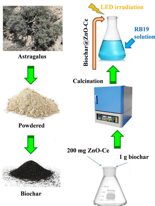
Figure 2. The preparation approach of the biochar@ZnO–Ce nanocatalyst and its utilization in RB19 dye removal.
