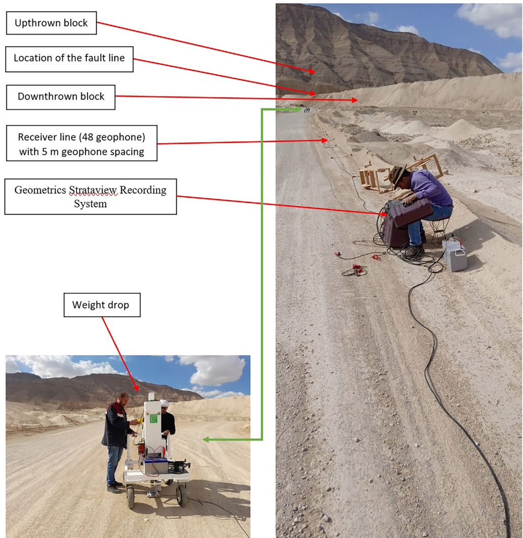
Figure 8. (a) Components of the acquisition system with an overview of the exposed Quaternary fault, (b) zoom in on the weight drop.
