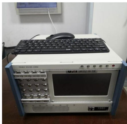
Figure 6. Super dynamic strain gauge test system.
