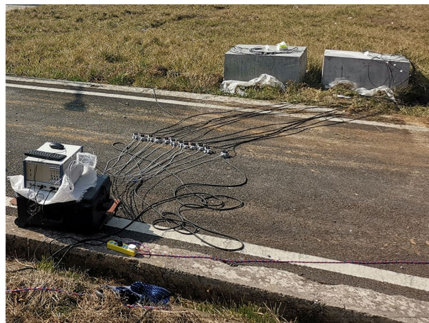
Figure 8. Super dynamic strain test system test diagram.
