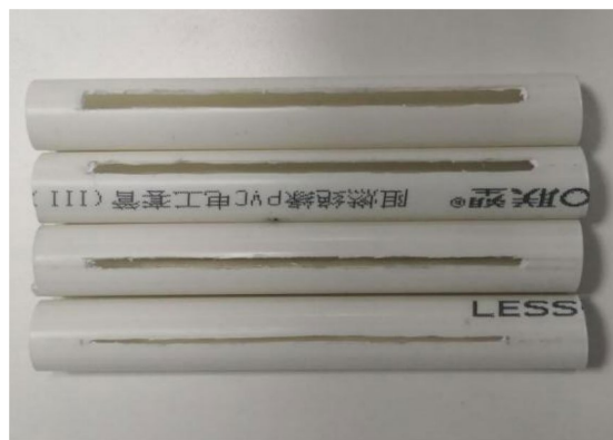
Figure 14. Four slit tubes with different slit angles.
