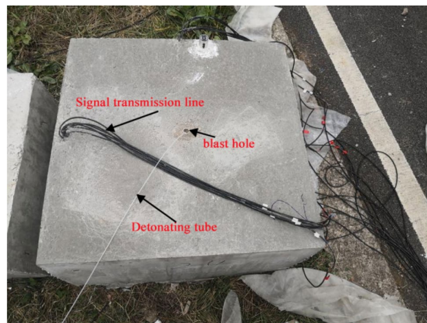
Figure 7. Charge model test block before blasting.
