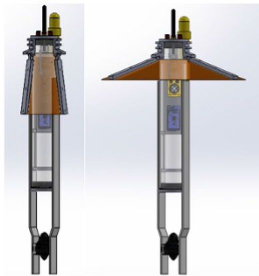
(a) An open and closed "umbrella" model of the floater used for jellyfish motion characteristics relative to the water current
