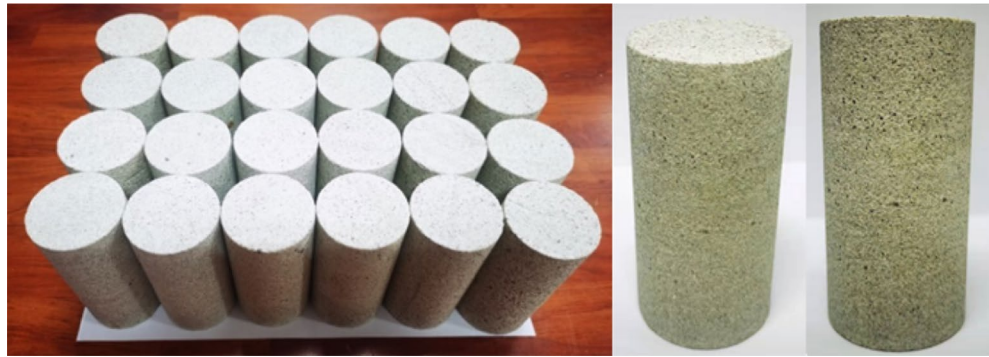
Figure 2. Rock white sandstone specimens for tests.
