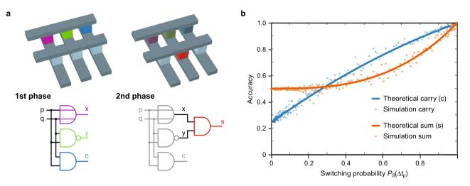
**Figure 5.** (a) The process of the arithmetic operation within the crossbar with the two phases to produce the sum and carry bits. (b) The theoretical and simulated outputs for the adder circuit.
