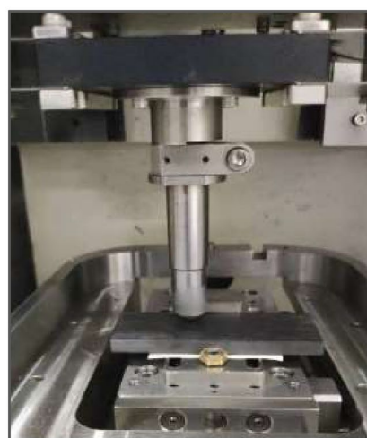
Figure 2. UMT-3 friction and wear tester. Figures were created using the Microsoft Visio software (version 2010) and SOLIDWORKS (version 2018).
