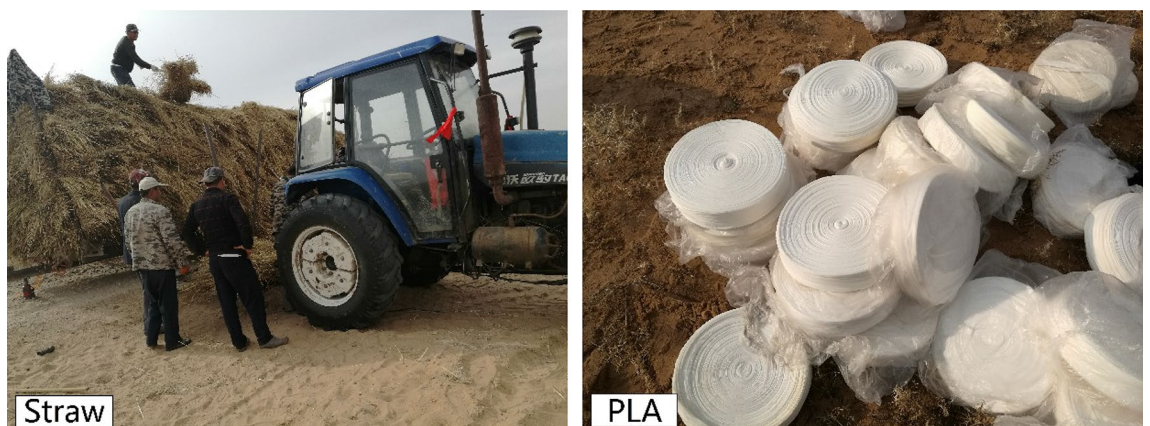
Figure 2. Sand barrier materials including wheat straw (left) and PLA tubing (right).
