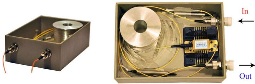
Figure 6. The optical module of the O-band BDFAs constructed utilizing unidirectional backward pumping configuration using a commercially available laser diode operating at 1.23 \mu\text{m} .
