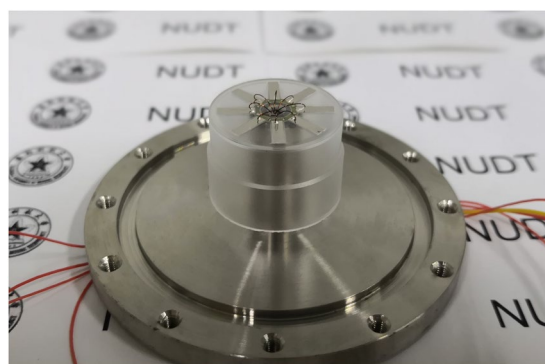
Figure 9. Ge02 fixed on the Invar base and conductor wires completed.
