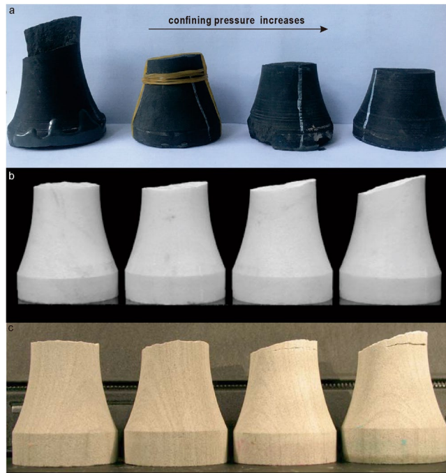
Figure 3. Fracture angle of Longmaxi Shale (a), Carrara Marble 20 (b), and Berea Sandstone 21 (c). From left to right, the fracture angles for marble and sandstone increase with confining stress. The fracture angle for the shale, on the contrast, decreases as confining stress increases.
