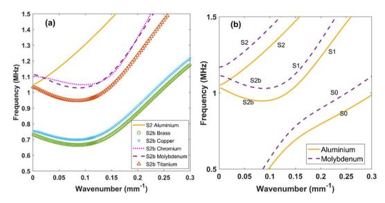
**Figure 1.** Lamb wave dispersion curves generated for a plate thickness of 3 mm. (a) Illustration of the  $S_2$  mode of Aluminium and  $S_{2b}$  mode of the other materials. (b) Intersection of  $S_2$  and  $S_{2b}$  mode of Aluminium and Molybdenum respectively at 1.09 MHz frequency.
