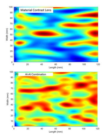
**Figure 4.** Top View. 2D scan representation obtained from experimentally monitored wave amplitude on the surface of plate across the interface. (a) Material contrast lens (b) Al-Al combination. Focusing is observed at 47 mm from the interface in material contrast lens compared to Al-Al combination.
