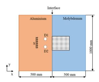
**Figure 7.** Schematic representation showing the configuration used to study the subwavelength imaging of defects using numerical simulations. S is the plane wave source, D1 & D2 are the defects, which are in subwavelength regime and placed near the interface of the material contrast lens. The dotted area shown on the Molybdenum side is the region selected for imaging of defects.
