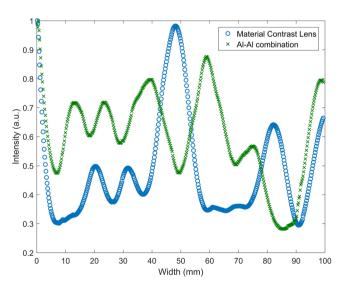
**Figure 5.** Plot showing the variation of the measured out-of-plane displacement amplitude along the width for material contrast lens compared with Al-Al combination.
