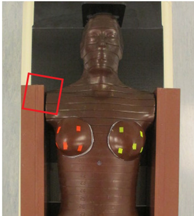
Figure 1. Female Alderson phantom with water equivalent slabs (thickness 8 cm) on each side mimicking the arms. TLD crystals were positioned on each breast as follows: two TLDs in each quadrant (one at the base and one at the surface), one in a borehole in the center of the breast and one at the papilla of the breast. The red (ipsilateral) and yellow (contralateral) marks show the locations of the TLDs at the surface of the breasts in relation to the Co-60 treatment field ( 12 \times 12 cm) of the right shoulder. Between the torso and the breasts white thermoplastic material with a thickness of 6 mm was added, where the TLDs at the base of the breast were inserted.
