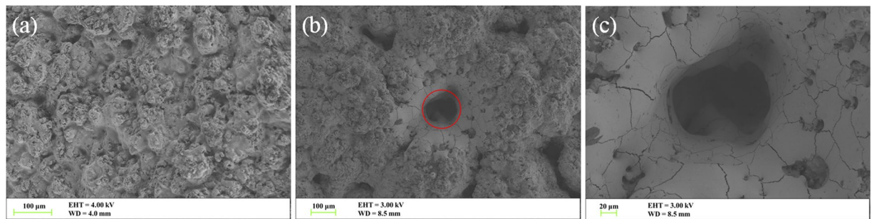
Figure 13. The typical surface views of the electrode with coating (a) before and (b) after LI BD tests. (c) Enlargement view of (b).
