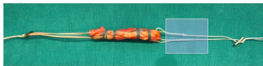
Figure 8. Shows the part of TightRope crossing; were the failure occurred most often.
