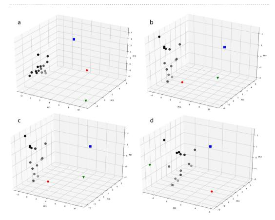
**Figure 3.** The PC scores of microstructures shown for the first four PCs: (**a**) PC1, PC2, and PC3; (**b**) PC1, PC2, and PC4; (**c**) PC1, PC3, and PC4; (**d**) PC2, PC3, and PC4. The gray scale symbols are the experimental microstructures, the blue square is the ideal SRB, the green upside down triangle is the ideal LAM, and the red polygon is the ideal RHN.
