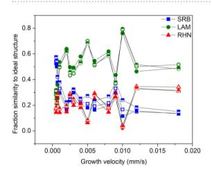
**Figure 5.** The fraction similarity to SRB, LAM, and RHN ploted versus solidification velocity. Filled symbols are fractions obtained from triangulated values in PCA, the empty symbols are the PLS regression results using all 19 attributes, and half-filled symbols show the results from a 9 attribute PLS regression.
