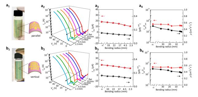
**Figure 5.** Typical photograph and schematic images, typical transfer curves,  $I_{ON}$ ,  $I_{OFP}$  mobility and  $I_{ON}/I_{OFF}$  of the device at strain bending ( $\mathbf{a_1}$ - $\mathbf{a_4}$ ) parallel and ( $\mathbf{b_1}$ - $\mathbf{b_4}$ ) vertical to channel length. The bending radius is from 3.3 to 0.23 cm.
