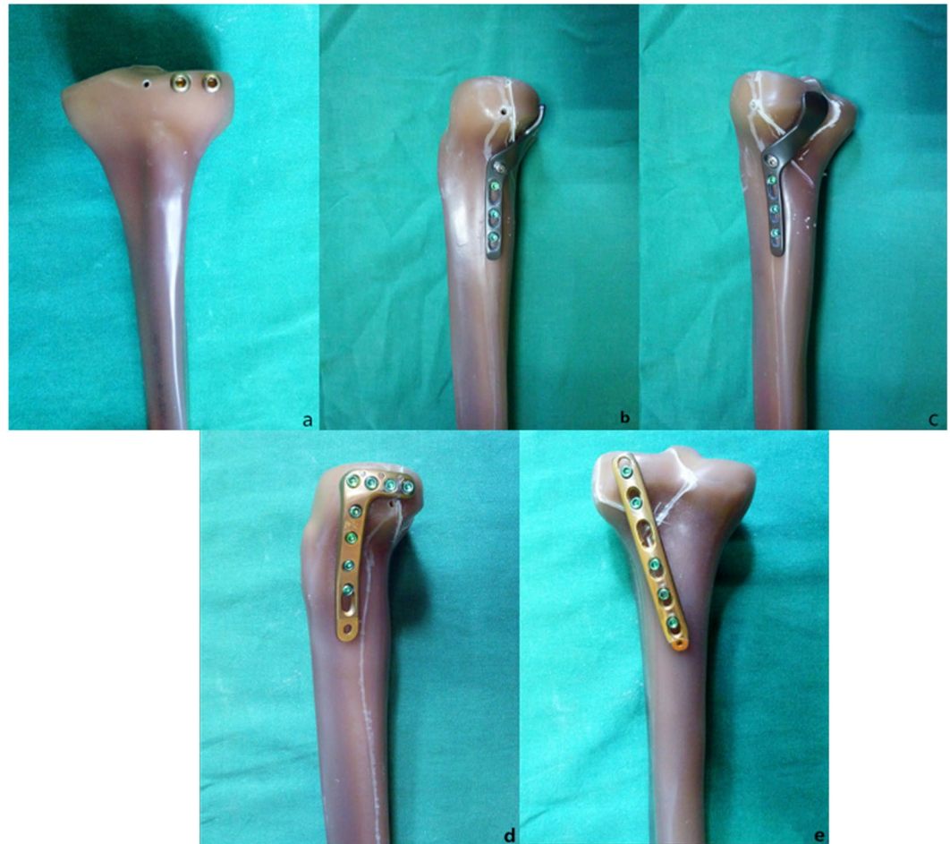
Figure 3. Implant types. (a) Two anterolateral 6.5-mm parallel lag screws, (b,c) Newly designed plate. (d) A 3.5-mm lateral anatomic locking plate. (e) A 3.5-mm six-hole posterolateral buttress plate.
