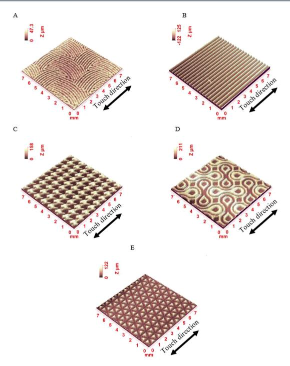
**Figure 4.** Confocal scans of five plastic sample topographies. The five plastic surfaces had the same stiffness but different textures with different tactile properties. The support material was PVC, and the printed material was UV light ink. The digital printer was the Mímaki brand with a resolution of 1,200 bpi.
