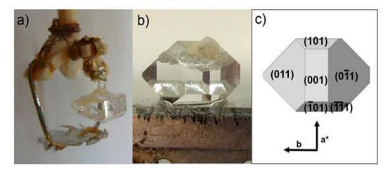
**Figure 1.** (a) As-grown single crystal of  $Ce^{3+}$ :KGdP and platinum stirrer, (b) As-grown single crystal of  $Ce^{3+}$ :KGdP and (c) Crystal scheme with the faces observed.
