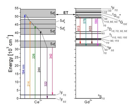
**Figure 4.** Energy levels diagram of  $Ce^{3+}$  and  $Gd^{3+}$  in  $KGd_{0.996}Ce_{0.004}(PO_3)_4$  and the emission mechanism. ET = Energy Transfer.
