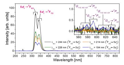
**Figure 3.** Optical emission spectra of  $KGd_{0.996}Ce_{0.004}(PO_3)_4$  under 244, 226, 214 and 194 nm excitation. Labels in purple (inset) indicate the transitions of  $Gd^{3+}$  and labels in pink those of  $Ce^{3+}$ .
