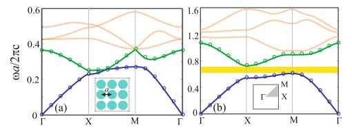
**Figure 1.** Band structures for the PhCs made of InSb (**a**) without and (**b**) with external magnetic field. The open circles represent the results (for the first two bands) calculated using the finite element method. The inset in (a) is a schematic of the PhC, and the inset in (b) is the first Brillouin zone. The radius of the InSb rods is r = 0.46a. The external magnetic field in (b) is  $B_0 = 0.9$  T (i.e.,  $\omega_c = 0.9\omega_p$ ).
