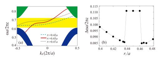
**Figure 6.** (a) Dispersion curves of the edge mode for the different radii  $r_1 = 0.42a$ , 0.45*a*, and 0.47*a*. (b) ROWP bandwidth as a function of the radius  $r_1$ . The other parameters are the same as those in Fig. 2.
