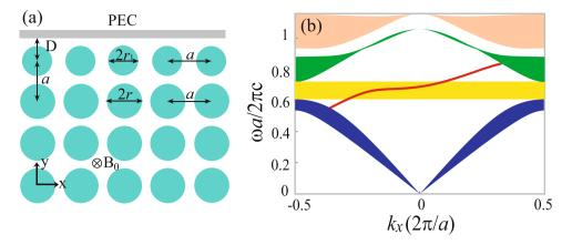
**Figure 2.** (a) Schematic of a PhC system for guiding robust one-way edge mode. The radius  $(r_1)$  of the InSb rods at the outmost row may be different from that (r) in the PhC. (b) Dispersion curve of the edge mode. The shaded rectangular area indicates the band gap of the PhC. Other three shaded areas represent the projected bands of the PhC along  $\Gamma - X$  direction. The parameters of the PhC are the same as in Fig. 1(b). D = 0.6a and  $r_1 = r = 0.46a$ .
