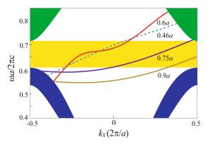
**Figure 7.** Dispersion curves of the edge mode for *D* = 0.46*a*, 0.6*a*, 0.75*a*, and 0.9*a*. The other parameters are the same as in Fig. 2.
