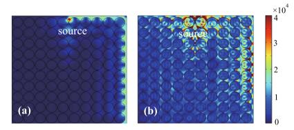
**Figure 4.** Simulated electric field amplitudes in a 90° bent guiding systems with (**a**)  $B_0 = 0.9$  T and (**b**)  $B_0 = 0$ . In (b), edge mode cannot be sustained by the PhC where the external magnetic field is removed. The other parameters of the systems are the same as in Fig. 2.
