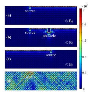
**Figure 3.** Simulated electric field amplitudes in the PhC systems with different external magnetic fields. (a)  $B_0 = 0.9$  T, (b)  $B_0 = 0.9$  T but with an obstacle, (c)  $B_0 = -0.9$  T, and (d)  $B_0 = 0$ . The obstacle in (b) is a metal slab of sizes  $0.97a \times 2a$  (i.e.,  $0.6\lambda \times 1.26\lambda$ ). In all cases, the source is a linear magnetic current located in the air layer and the frequency is 3.1 THz. The other parameters of the PhC systems are the same as in Fig. 2.
