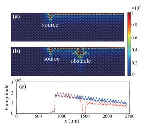
**Figure 5.** Simulated electric field amplitudes in the lossy systems (**a**) without and (**b**) with obstacle. (**c**) Electric field amplitudes on the central line of the air layer in the system. The solid and dotted lines correspond to the relevant results in (a,b), respectively. The loss parameter is  $\nu = 10^{-3}\omega_p$ , and the other parameters are the same as in Fig. 3(a,b).
