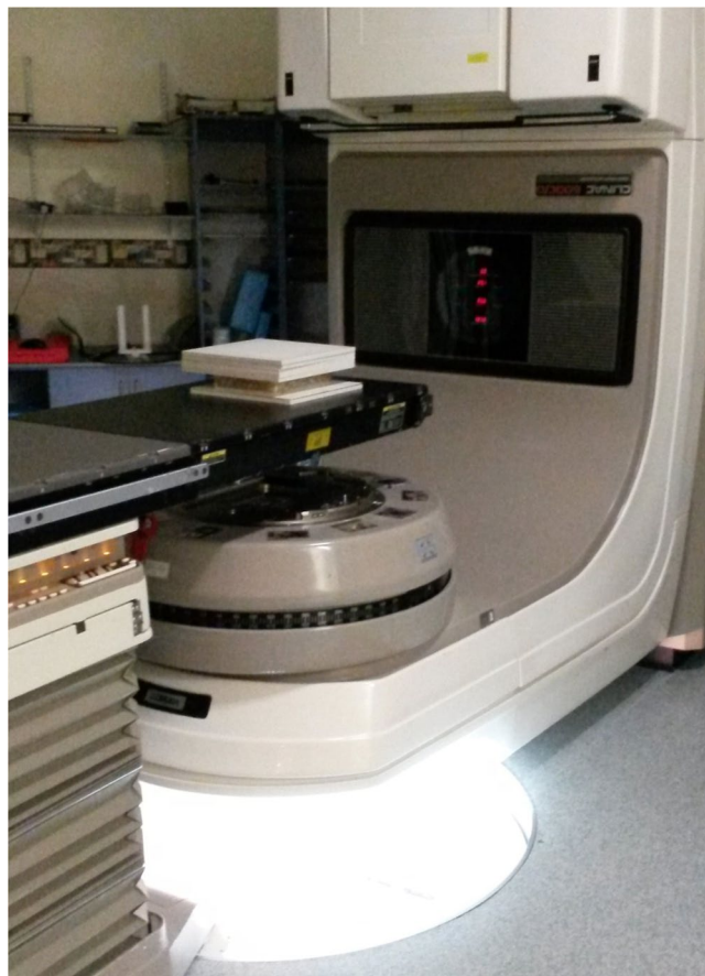
Figure 2. Irradiation setup for MTT experiments using a 6 MV beam from a Varian 600CD linear accelerator.
