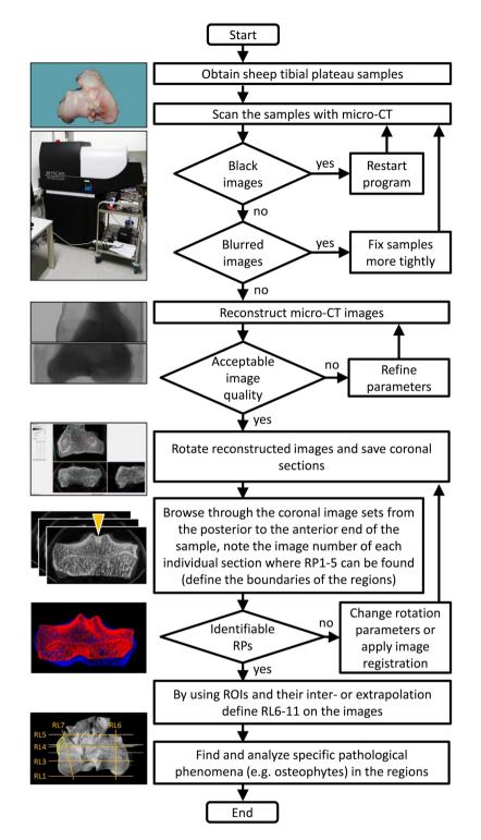
**Figure 8.** Flowchart diagram of the workflow to identify specific pathological phenomena. The individual steps required for obtaining micro-CT image sets, and their analysis for determining the location of specific pathological phenomena including osteophytes using the newly defined regions are illustrated. A particularly important step is the uniform rotation of the reconstructed images.
