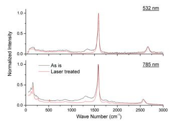
**Figure 5.** Raman spectra where black is the as-is 'before' and red is the atmospheric laser processed material 'after'. After laser processing, this shows reduction of the D peak located near 1320 cm<sup>-1</sup> (785 nm laser line) or near D peak removal (532 nm laser line). Radial breathing modes are preserved despite flash oxidation vaporizing a significant majority of the carbon material.
