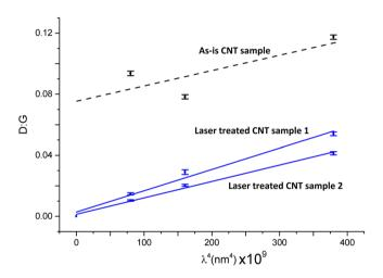
**Figure 6.** Raman spectroscopy's D:G of is plotted against  $\lambda^4$  the Raman excitation wavelength. Only after the laser process, with removal of multiwall CNTs and malformed carbons, does D:G  $\propto \lambda^4$ , which is the typical response of graphene and graphite.
