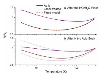
**Figure 7.** Resistance versus temperature plots, normalized by the room temperature resistance, for as-is material (black) and laser treated material (blue). Dashed red lines are the best fit models. (a) After the HCl/ $\rm H_2O$  wash and (b), after nitric acid treatment. Resistance values are normalized by the room temperature resistance  $R_0$ . For clarity, the grey ghost plots depict where the traces were before nitric acid treatment.
