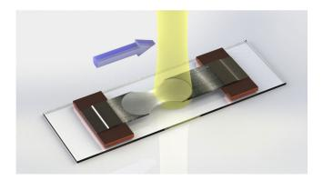
**Figure 1.** Depiction of the atmospheric laser process, with the yellow beam showing translational movement. FWCNT textile must be elevated off the substrate by suspending it from its ends where a laser sweeps across the surface leading to selective oxidation.
