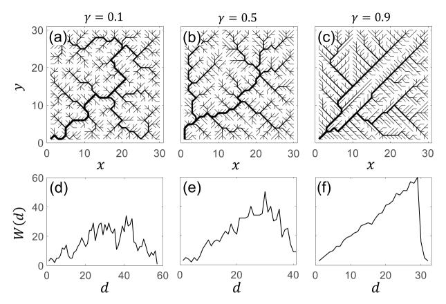
**Figure 4.** (a-c) Examples of optimal channel networks generated with  $\gamma = 0.1$ , 0.5 and 0.9 respectively. (d-f) The associated width functions. As can be seen from this figure, with increasing  $\gamma$ , the maximum channel length  $d_{max}$  decreases.
