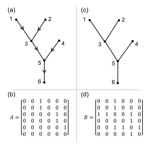
**Figure 1.** An exemplary stream network and its adjacency matrix. (a) The directed graph representation, (b) the asymmetric adjacency matrix A, (c) the undirected graph representation, and (d) the symmetric adjacency matrix B.
