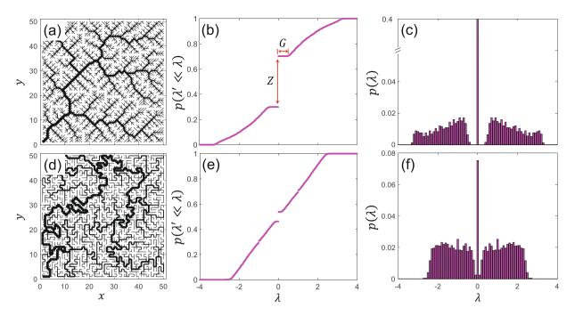
**Figure 2.** (a) A river network generated with an optimal channel network model on a  $50 \times 50$  square lattice. (b,c) The cumulative density function (cdf) and the probability density function (pdf) of the associated adjacency matrix eigenvalue spectrum. (d) A randomly generated spanning tree on the same lattice and (e,f) its associated cdf and pdf. *G* and *Z* in (b) represent spectral gap and nullity, respectively.
