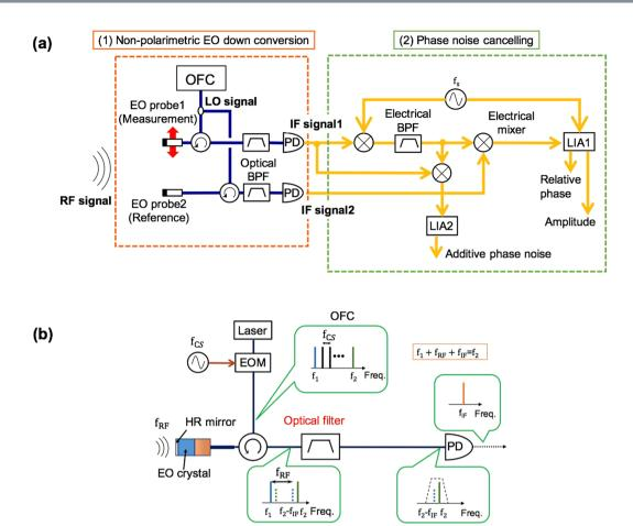
**Figure 2.** Basic configuration of the measurement setup. (**a**) System block diagram and (**b**) principle of the non-polarimetric EO frequency down conversion.
