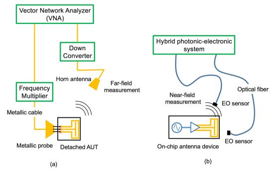
**Figure 1.** Comparison of the conventional and proposed measurement schemes. (**a**) Conventional system using a network analyzer and the (**b**) proposed system.
