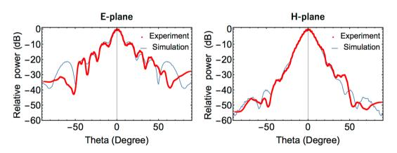
Figure 5. Radiation patterns of the horn antenna calculated from the measured near-field.
