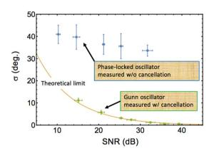
Figure 3. Relationship between the phase standard deviation and the amplitude SNR.
