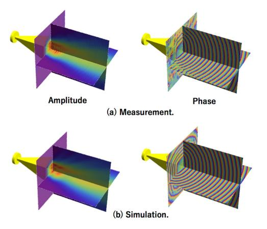
**Figure 4.** Amplitude and phase distribution of the mm-wave emitted by a horn antenna. The signal source is a free-running Gunn oscillator. (**a**) Measured results and (**b**) simulated results. Note: The pyramidal horn antennas are simulation models.
