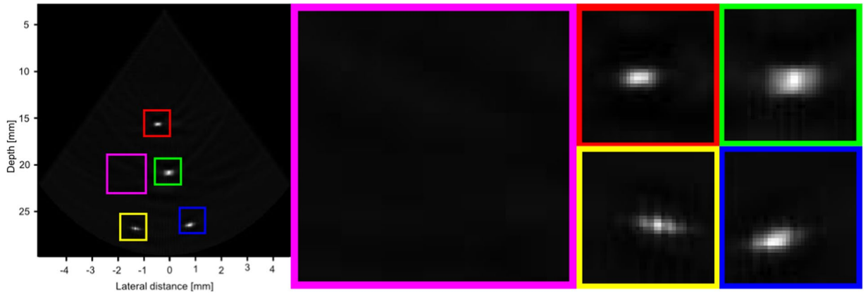
Figure 14. A closer look at the EG-CRCUIS reconstruction. Better noise suppression was achieved. 40 dB is the dynamic range.
