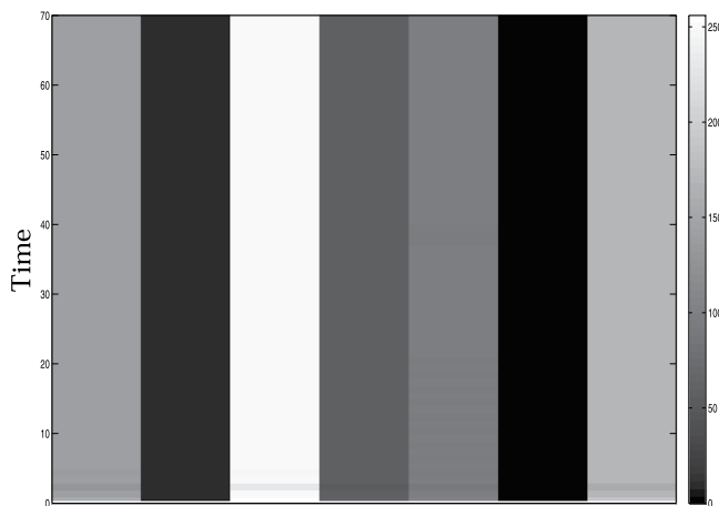
Figure 3. Splined (in x direction) image of one dimensional pattern \{142, 10, 200, 58, 96, 3, 171\} decoded from the globally coupled Rulkov maps with \alpha = 3.5 , \beta = 0.0005 , \sigma = 0.001 and N = 9 .
