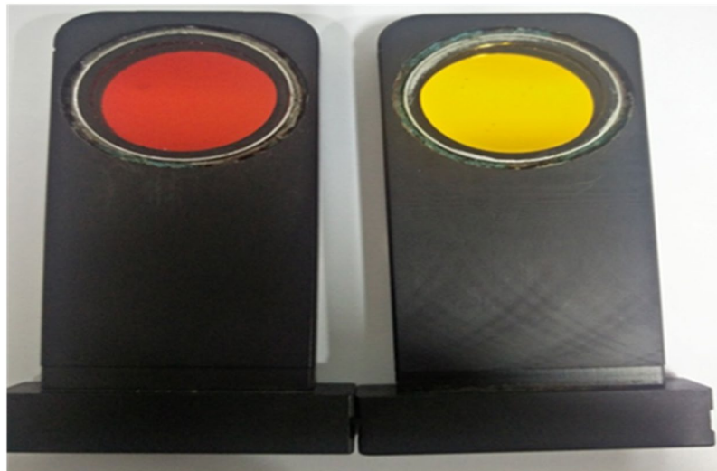
Figure 1. Manual Filters of wavelength 570 and 600 nm used for capturing the retinal images.
