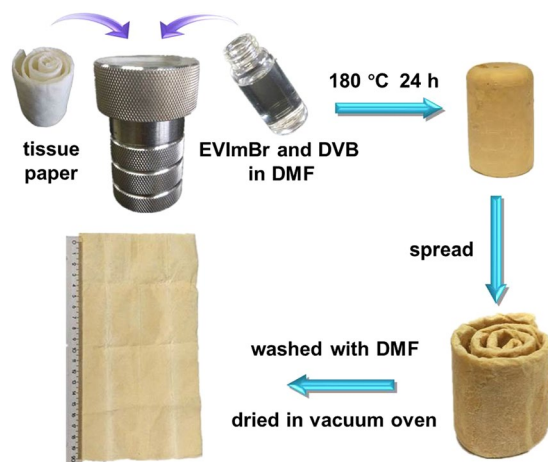
Figure 1. The schematic illustration of the preparation of PPHMs via solvothermal copolymerization of EVImBr and DVB in DMF in the presence of tissue paper in an autoclave.
