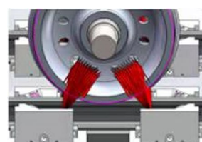
Fig. 2 The lower left corner is a schematic diagram of the process of taking a wheel pair laser light strip with a CCD camera. The original image obtained is manually annotated and repaired, and the centerline is extracted. The annotated centerline image is obtained by adding the images.
