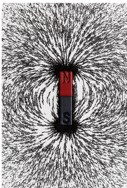
Iron filings following the magnetic field lines of a bar magnet. Credit: Alchemy/Alamy Stock Photo
