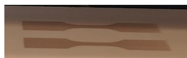
Fig. 7 | Red color of activating fusing agent visible on powder bed before fusing. X1 and X2 dog bones printed show the color of the AFA immediately after being deposited on the powder bed, before fusing and reduction turning colorless.
